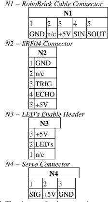
3. The pin–outs for the two sockets are listed below:
