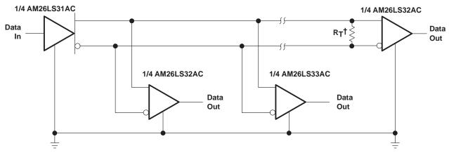
$^{\dagger}$  R<sub>T</sub> equals the characteristic impedance of the line.
