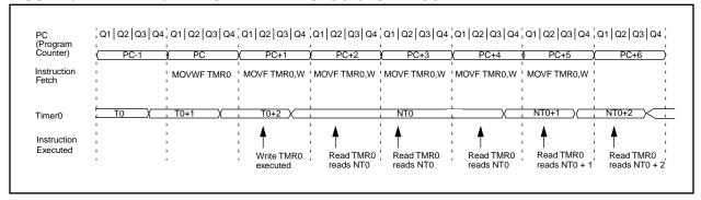
FIGURE 6-3: TIMERO TIMING: INTERNAL CLOCK/PRESCALE 1:2
