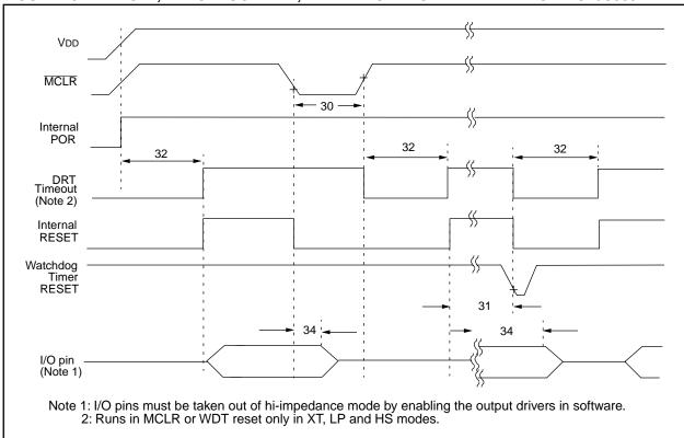
FIGURE 10-4: RESET, WATCHDOG TIMER, AND DEVICE RESET TIMER TIMING - PIC16C505
