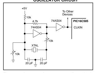
Figure 7-5 shows a series resonant oscillator circuit. This circuit is also designed to use the fundamental frequency of the crystal. The inverter performs a 180-degree phase shift in a series resonant oscillator circuit. The 330  $\Omega$  resistors provide the negative feedback to bias the inverters in their linear region.
