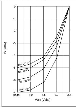
FIGURE 11-6: IOH vs. VOH, VDD = 5.5 V
