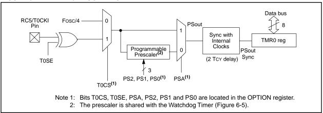
FIGURE 6-2: TIMERO TIMING: INTERNAL CLOCK/NO PRESCALE
