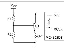
This brown-out circuit is less expensive, although less accurate. Transistor Q1 turns off when VDD is below a certain level such that:
