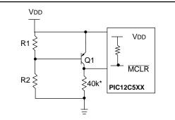
This brown-out circuit is less expensive, although less accurate. Transistor Q1 turns off when VDD is below a certain level such that:
