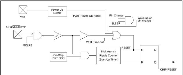
FIGURE 7-9: TIME-OUT SEQUENCE ON POWER-UP (MCLR PULLED LOW)
