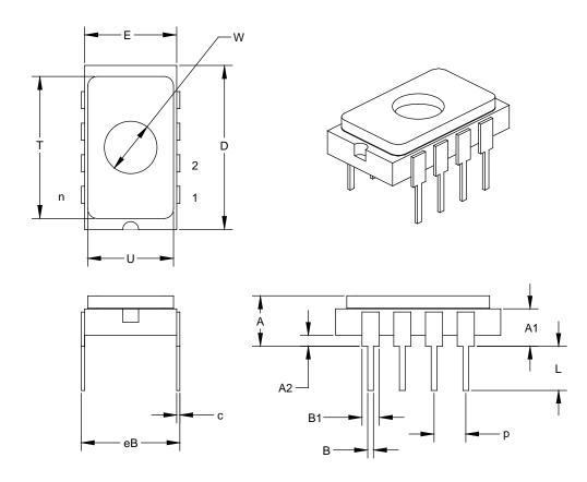
Package Type: K04-084 8-Lead Ceramic Side Brazed Dual In-line with Window (JW) – 300 mil
