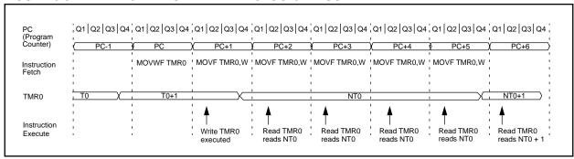
FIGURE 6-4: TIMERO INTERRUPT TIMING
