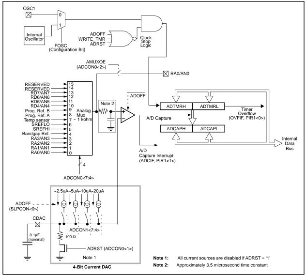
FIGURE 8-2: EXAMPLE A/D CONVERSION CYCLE
