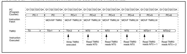
FIGURE 6-3: TIMER0 TIMING: INTERNAL CLOCK/PRESCALE 1:2
