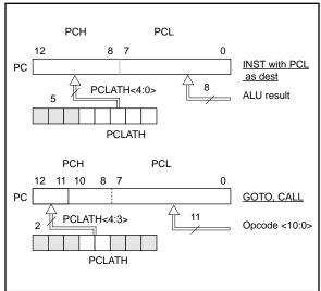
Note: On POR, the contents of the PCLATH register are unknown. The PCLATH should be initialized before a CALL, GOTO, or any instruction that modifies the PCL register is executed.
