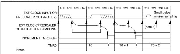
FIGURE 6-5: TIMERO TIMING WITH EXTERNAL CLOCK
