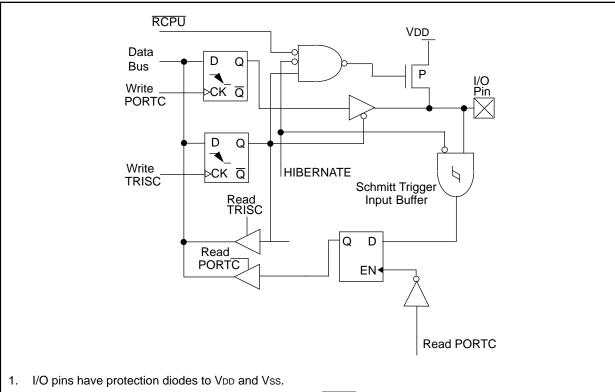
FIGURE 5-5: BLOCK DIAGRAM OF PORTC<3:0> PINS
