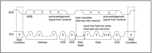
When a master does not wish to relinquish the bus (by generating a STOP condition), a repeated START (Sr) must be generated. This condition is identical to the START (SDA goes high-to-low while SCL is high), but occurs after a data transfer acknowledge pulse (not the
