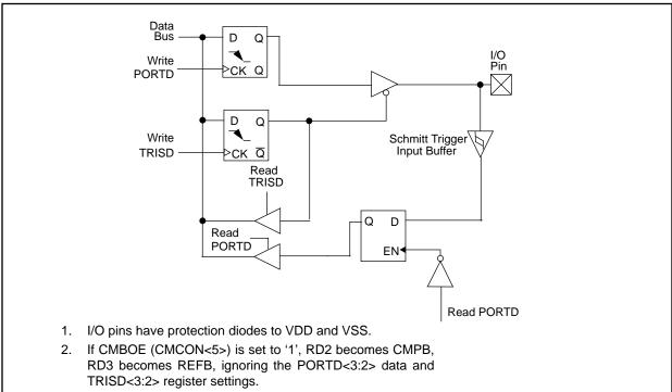
FIGURE 5-10: BLOCK DIAGRAM OF PORTD<1:0> PINS
