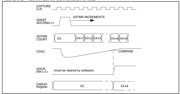
FIGURE 8-3: A/D CAPTURE TIMER (LOW BYTE)
