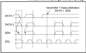
FIGURE 7-12: I<sup>2</sup>C CLOCK SYNCHRONIZATION
