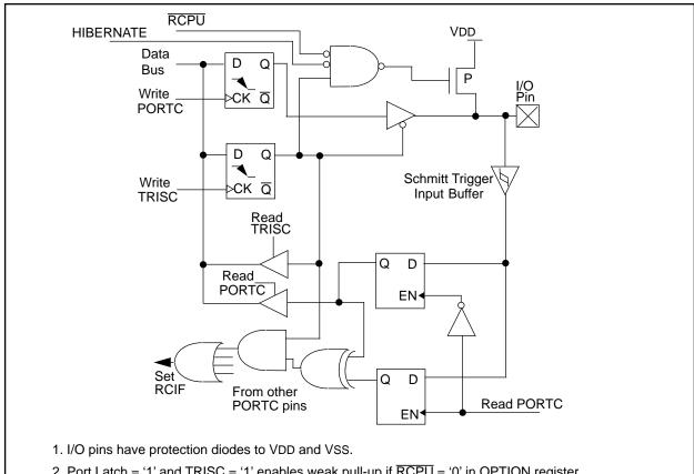
2. Port Latch = '1' and TRISC = '1' enables weak pull-up if  $\overline{RCPU}$  = '0' in OPTION register.
