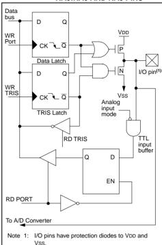
FIGURE 3-2: BLOCK DIAGRAM OF RA4/ T0CKI PIN
