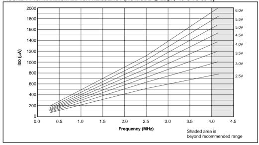
FIGURE 14-14: TYPICAL IDD vs. FREQUENCY (RC MODE @ 100 pF, 25°C)
