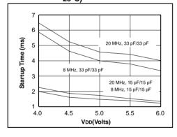
FIGURE 14-24: TYPICAL XTAL STARTUP TIME vs. VDD (XT MODE, 25°C)
