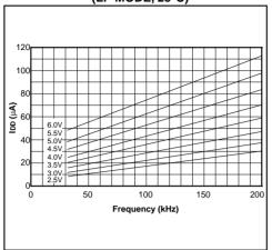
FIGURE 14-26: MAXIMUM IDD vs. FREQUENCY (LP MODE, 85°C TO -40°C)
