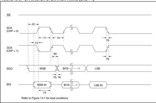
FIGURE 13-10: SPI SLAVE MODE TIMING (CKE = 0)
