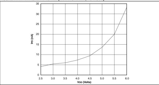
FIGURE 14-2: MAXIMUM IPD vs. VDD (WDT DISABLED, RC MODE)
