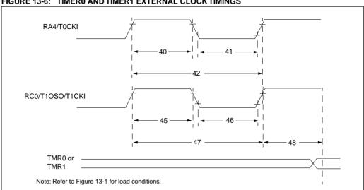
FIGURE 13-6: TIMERO AND TIMER1 EXTERNAL CLOCK TIMINGS
