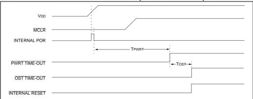
FIGURE 11-9: TIME-OUT SEQUENCE ON POWER-UP (MCLR NOT TIED TO VDD): CASE 2
