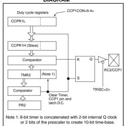
A PWM output (Figure 7-5) has a time base (period) and a time that the output stays high (duty cycle). The frequency of the PWM is the inverse of the period (1/period).
