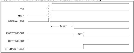
FIGURE 11-8: TIME-OUT SEQUENCE ON POWER-UP (MCLR NOT TIED TO VDD): CASE 1
