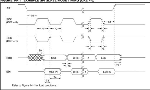
FIGURE 14-11: EXAMPLE SPI SLAVE MODE TIMING (CKE = 0)
