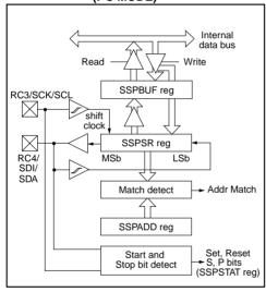
The SSP module has five registers for I<sup>2</sup>C operation. These are the:
