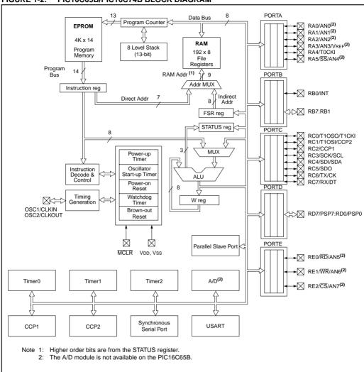
FIGURE 1-2: PIC16C65B/PIC16C74B BLOCK DIAGRAM
