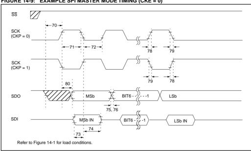
FIGURE 14-9: EXAMPLE SPI MASTER MODE TIMING (CKE = 0)
