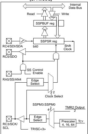
To enable the serial port, SSP enable bit, SSPEN (SSPCON<5>) must be set. To reset or reconfigure SPI mode, clear bit SSPEN, re-initialize the SSPCON register, and then set bit SSPEN. This configures the SDI, SDO, SCK, and SS pins as serial port pins. For the pins to behave as the serial port function, they must have their data direction bits (in the TRISC register) appropriately programmed. That is:
