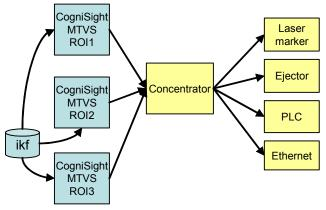
Multiple CogniSight MTVS adjusted with different focal planes (f3>f2>f1) using different ROI (ROI3<ROI2<ROI1), same knowledge file trained at a mid-range focal length, a result concentrator looking for the MTVS which will recognize the object with the highest confidence level when the latter enters the filed of view.
