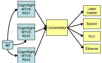
Multiple CogniSight MTVS installed to cover a continuous field of view at a same focal plane, same knowledge file trained to recognize a good texture, a result concentrator programmed to generate an "anomaly" signal if at least one MTVS does not recognize a good texture.
