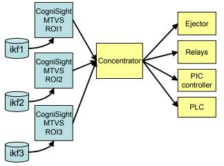
On a factory floor, CogniSight MTVS can be interfaced with an ejector to reject or divert parts, with a PC station to generate statistical report about the production and, if needed, record the images of parts with a certain type of defect.
