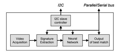
The neurons are taught what to recognize by learning examples. They are capable of generating models automatically as new examples are shown. The contents of the neurons constitutes a knowledge which can be saved. A knowledge can be build "live" on the board or loaded from an existing file or memory.
